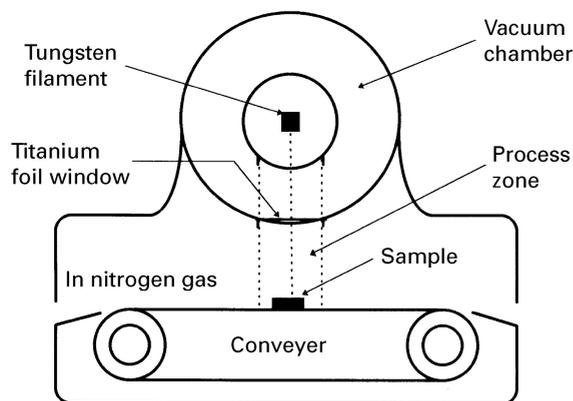
Figure 1 Schematic diagram of the electrocurtain processor.
