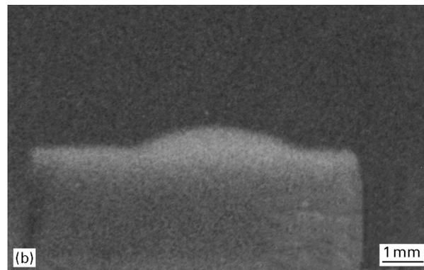
Figure 2 Photographs of a sessile drop of water on apatite ceramics, (a) before, and (b) after electron-beam irradiation.
