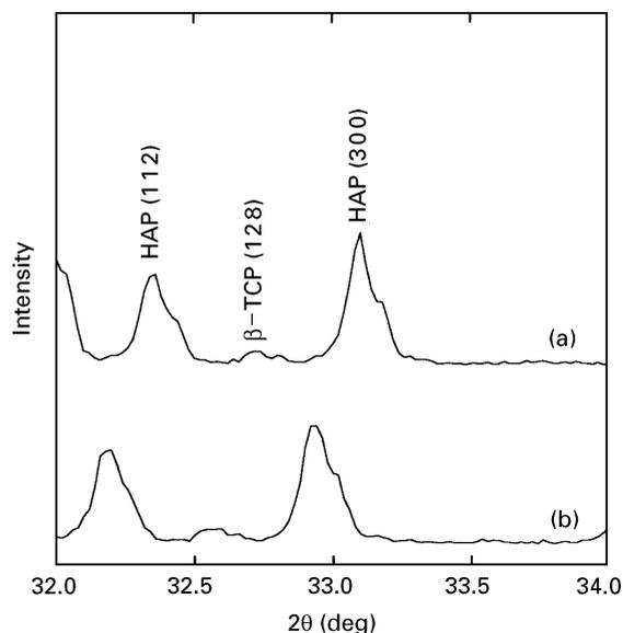
Figure 4 X-ray diffraction patterns of apatite ceramics (a) before and (b) after electron beam irradiation.
