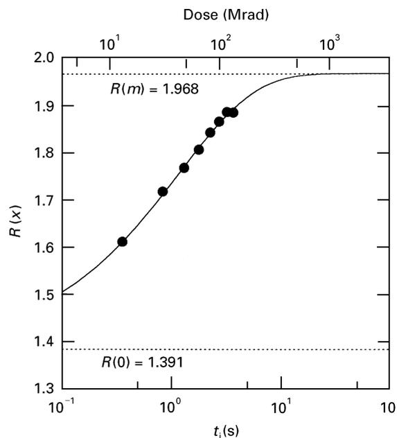
Figure 3 Change in reduced interfacial energy,  $R(x)$ , with electron-beam irradiation time,  $t_i$ .
